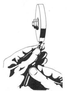
Fig. 14. Drill Grinding. The beginning of the movement seen from above.
