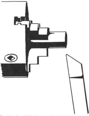
Fig. 20. A tool this shape can be used for facing and turning at the same setting.
