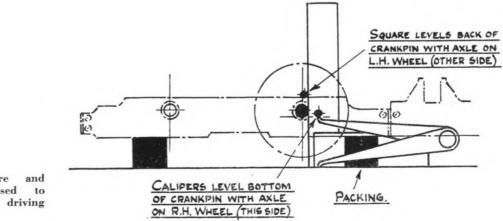
Fig. 49. How the square and calipers are used to "quarter" the driving wheels.
