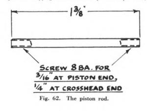
and "Tapping in the Lathe," p.206, Nov. 1952. Put a *slight* countersink in the end of the hole, and part off the piston to finished thickness. Alternatively saw it off as square as you can, and screw it temporarily on to the piston rod with this side outwards, hold the rod in the 3-jaw chuck with the side of the piston flat against the fronts of the jaws, and *carefully* face the piston down to size.
