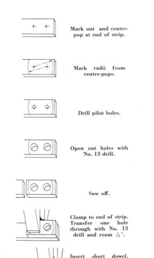
Insert short dowel, shift clamp and transfer other hole No. 13 and ream 3/16 in.
