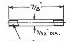
SCREW 8 B.A. FOR 1/4" EACH END. Fig. 83. The Valve Rod.
