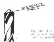
Fig. 18. The cutting edges of the drill must be "backed off" to provide clearance.
