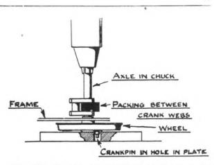
Fig. 48. Pressing the left-hand wheel on to the short end of the driving axle in the drilling machine.
