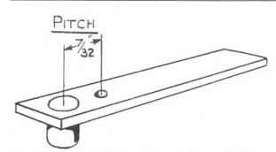
Fig. 31. Jig for drilling crankpin holes in wheels.
