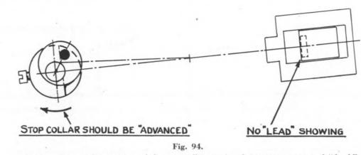
Adjusting the angular position of the stop-collar to give the correct amount of "lead." The crank is not shown, but is assumed to be in the back dead centre position, and the engine is running forwards.
