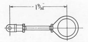
Fig. 85. Assembly of valve rod and eccentric strap.
