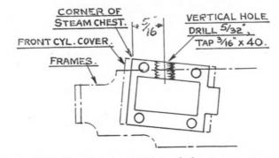
Fig. 76. Showing the position of the steam entry hole in the steam-chest, drilled with the cylinderblock in the frames. The valve and spindle should not be in place in the steam-chest while this is being done, and next time the block is removed from the frames the burrs should be cleaned off the inside.
