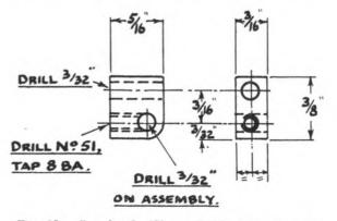
Fig. 63. Crosshead. (Shown finished but the crosshead pin hole is *not* drilled at this stage).
