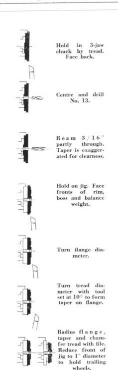
Fig. 30. Sequence of operations for turning wheel castings.
