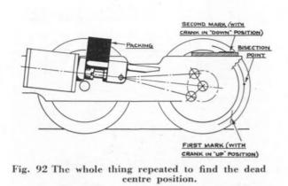
The process is now repeated for front dead-centre, using this time 3 in, of packing between the crosshead and cylinder cover (Fig. 92.). Your "marking-off" plate should, of course, be preserved in your box of "Aladdin"
