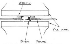
Fig. 21. Pressing the axle bush into the frame.
