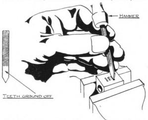
Fig. 52. A port-cutting chisel made from a broken piece of flat file and the chisel in use.
