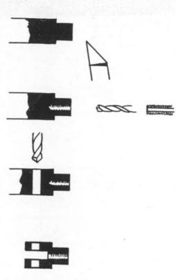
Fig. 82. Sequence of operations for making the Valve spindle fork-end.
