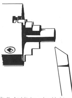
Fig. 20. A tool this shape can be used for facing and turning at the same setting.
