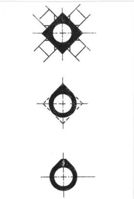
Fig. 41. Sequence of operations for making eccentric strap. Drawn full size. From top to bottom :
