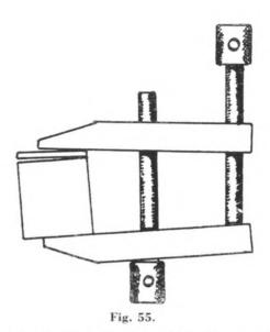
Keep the jaws of the toolmaker's clamp parallel --not like this!
