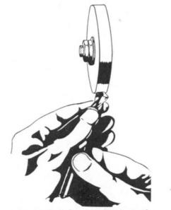
Fig. 14. Drill Grinding. The beginning of the movement seen from above.
