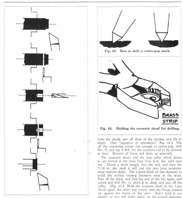
Fig. 42. Sequence of operations for turning eccentric sheaf and stop collar. From top to bottom :
