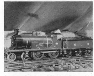
Coarse standard Gauge O Highland Railway 4-4-0 Loco. No. 12 "Ben Hope" of the small "Ben" class. Body and chassis built by the author and fitted with Walker Romford type mechanism. The loco. has since been rebuilt as "Ben Alder" No. 2. (The last of the class.)
