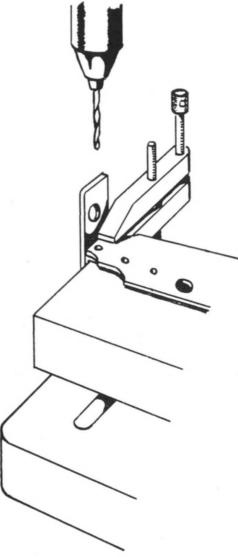
Fig. 8. Transferring screw holes from frame to angle bracket.
