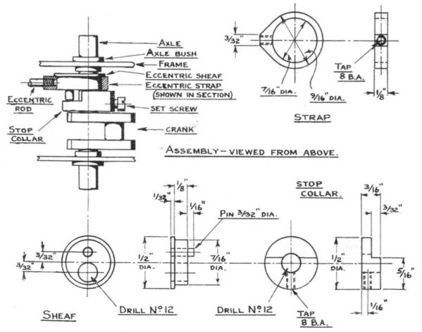
Fig. 39. The valve gear and its components.
