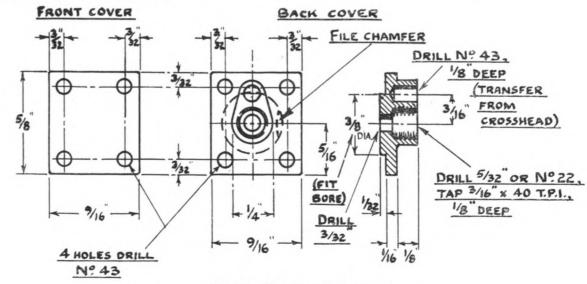
Fig. 54. The two cylinder covers
