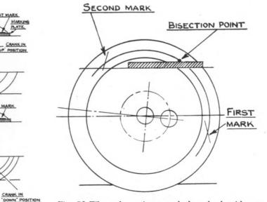
Fig. 91 When the point round the wheel mid-way between the two marks is placed against the marking plate, the crank is exactly on back "dead centre."
