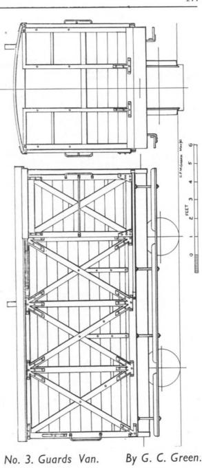
There are differences between the present form of the van and its condition in 1903, particularly in the pattern of outside framing for the body, and in the sliding doors. The 'Railway Magazine' photograph shows a conventional type of van with an open verandah leading to the van body through a hinged door.
