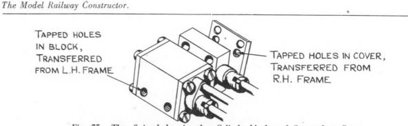
Fig. 75. The fixing-holes in the Cylinder-block and Steam-chest Cover.
