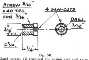
Gland screws (2 required for piston rod and valve spindle).
