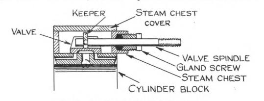
Fig. 73. Assembly of the Valve in the Steam-chest,
