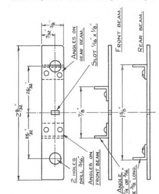
Fig. 5. Buffer Beams. Below: Photo-M. W. Earley.
