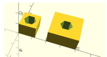
In OpenScad, the packaging device is called a module. It must have a name, and in parentheses a (possibly empty) list of parameters. Following that the *body* of the module is written within braces { }.
