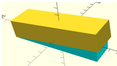
Finally, we 'subtract' the slanted cuboid from the original one to form the wedge:
