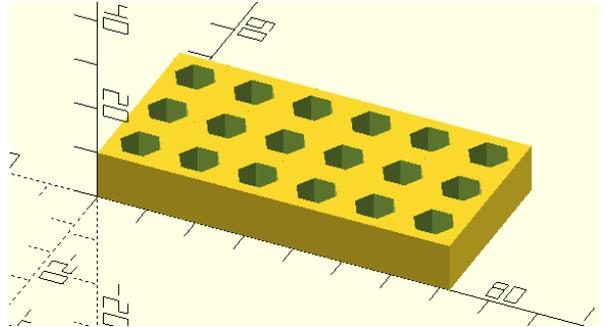
The starting point for this design in a 'cylinder' with six sides, which we construct by specifying `$fn=6` as part of the cylinder command. The 'diameter' of the hexagon (8.3mm) is slightly larger than the shank of a standard hex bit.
