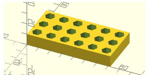
This new module has three parameters which set the size of the tray in terms of the number of bits it can accommodate in the X and Y directions, and the spacing between the holes. The defaults are for a 6x3 tray with 12mm between holes.
