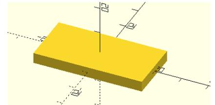
We make the curved ends by taking the *intersection* between a cylinder and the plate:
