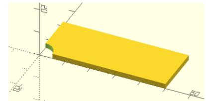
Objects can be moved about in space using the `translate()` operation. In OpenSCAD, points in space are specified using a *vector* which is written as a coordinate triple in square brackets: `[x, y, z]`.
