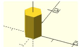
By subtracting this hex block from a cuboid, we get the basic building block of the bit tray:
