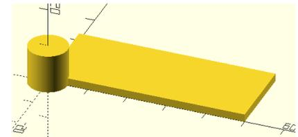
Objects can be ‘subtracted’ from one another using the `difference()` operation. If we write
