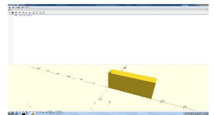
8. Click on the 3D preview window and try rotating and panning by click-and-dragging the left and right buttons. You can zoom in and out using your mouse wheel, or by using the
