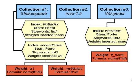
FIGURE 1: Concepts of indexing subsystem.
