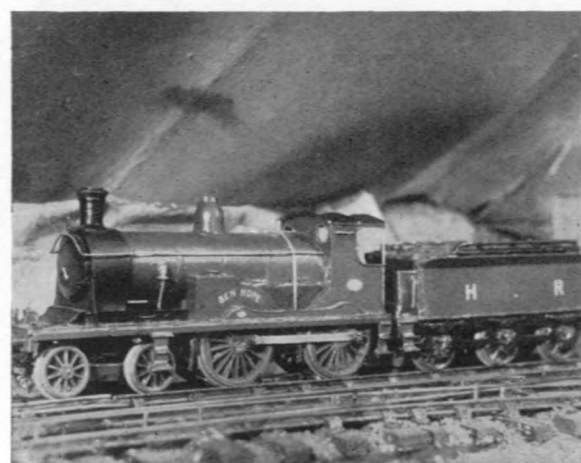
Coarse standard Gauge O Highland Railway 4-4-0 Loco. No. 12 "Ben Hope" of the small "Ben" class. Body and chassis built by the author and fitted with Walker Romford type mechanism. The loco. has since been rebuilt as "Ben Alder" No. 2. (The last of the class.)
