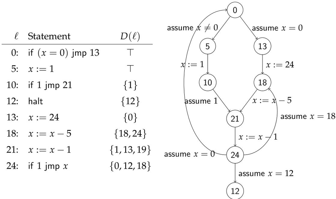
Figure 3.1: Control flow reconstruction example: IL program, final data flow information, and reconstructed control flow automaton.
