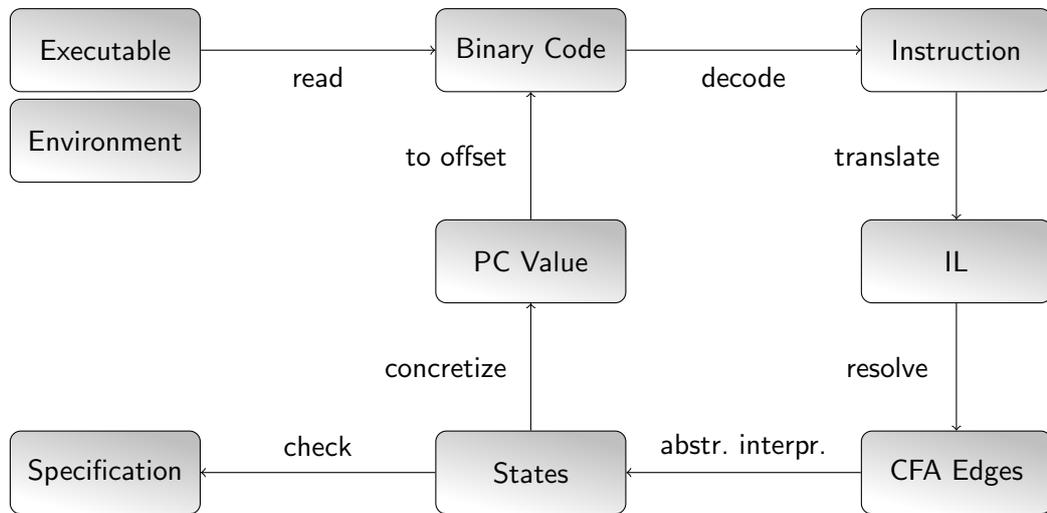
Figure 5.1: Unified disassembly and analysis architecture.
