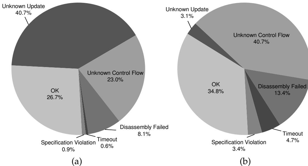
Figure 6.2: Results of analyzing 322 driver binaries from a standard Windows XP machine (a) using standard settings and (b) when ignoring weak updates.
