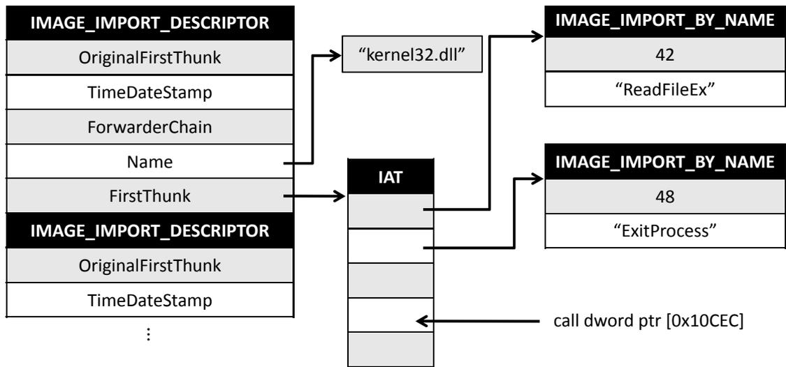
Figure 5.4: Dynamic linking in Windows PE files. The loader overwrites the Import Address Table (IAT) with the correct function entry points (adapted from [112]).
