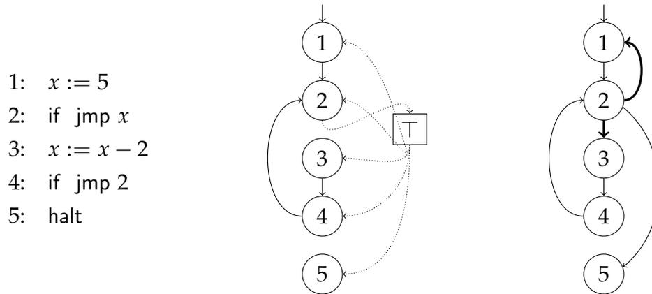
Figure 3.4: Adding an unknown node ( $\top$ ) with unlabeled edges leads to additional possible values for  $x$  at the indirect jump.
