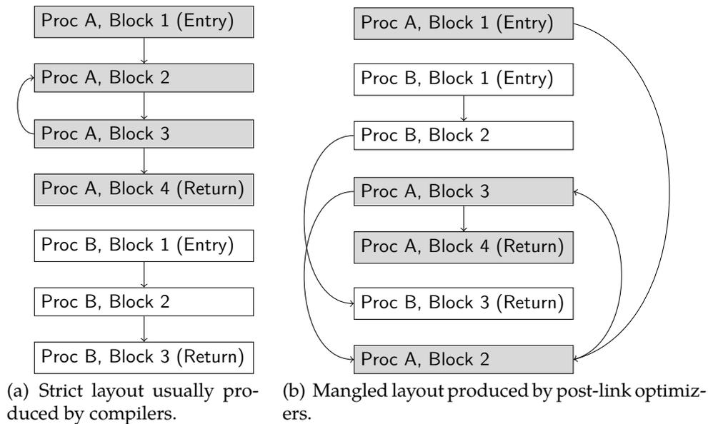
Figure 1.1: Example of possible procedure layouts in an executable.
