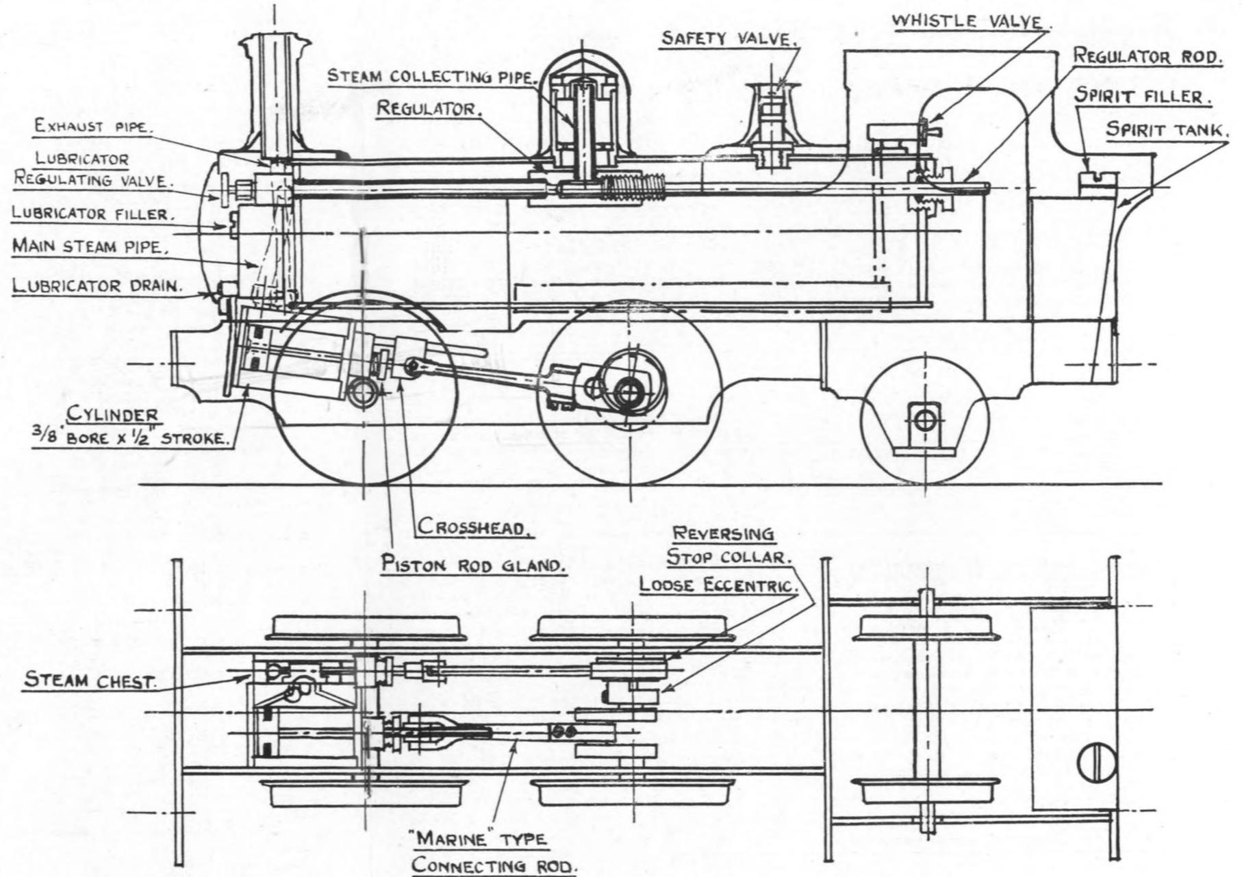
General arrangement of Gauge 0 steam loco—not to scale.
