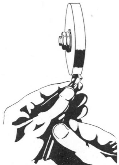
Fig. 14. Drill Grinding. The beginning of the movement seen from above.
