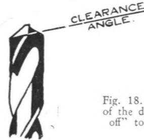
Fig. 18. The cutting edges of the drill must be "backed off" to provide clearance.
