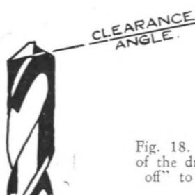
Fig. 18. The cutting edges of the drill must be "backed off" to provide clearance.
