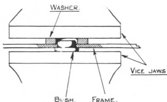
Fig. 21. Pressing the axle bush into the frame.
