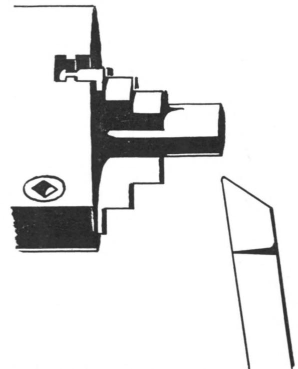
Fig. 20. A tool this shape can be used for facing and turning at the same setting.
