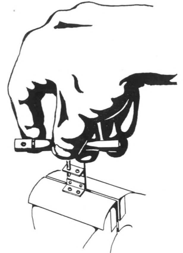
Fig. 9. Tapping the angle brackets.
