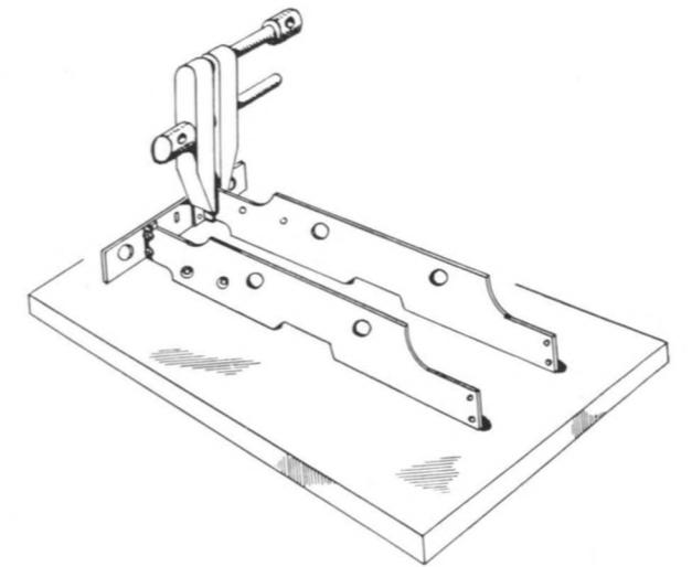
Fig. 10. Square up the frame assembly on the surface plate at all stages.
