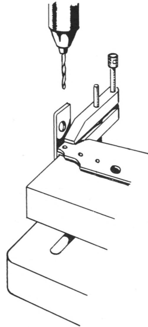
Fig. 8. Transferring screw holes from frame to angle bracket.
