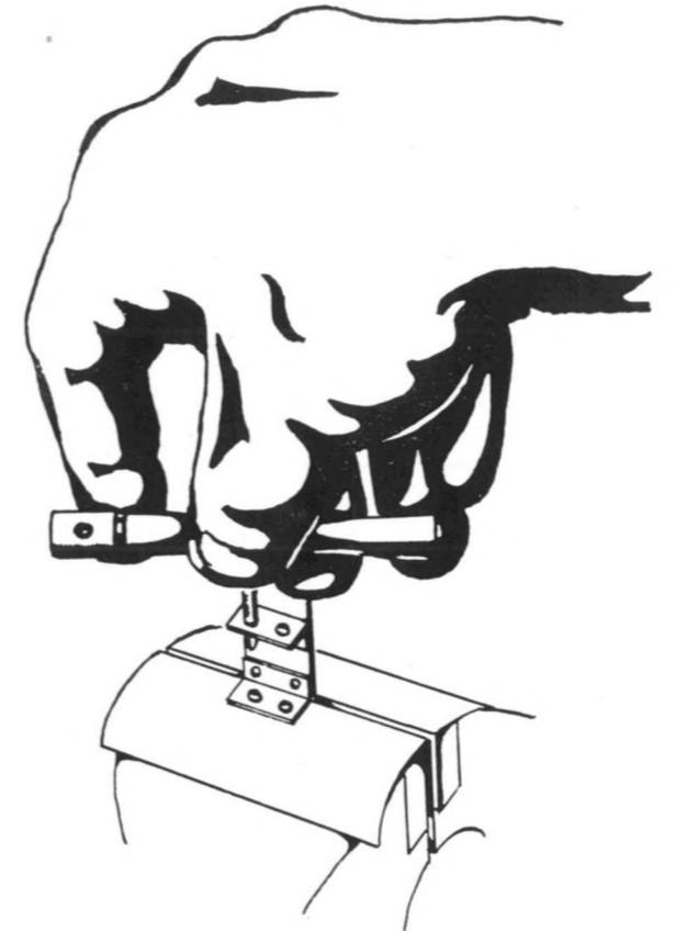
Fig. 9. Tapping the angle brackets.
