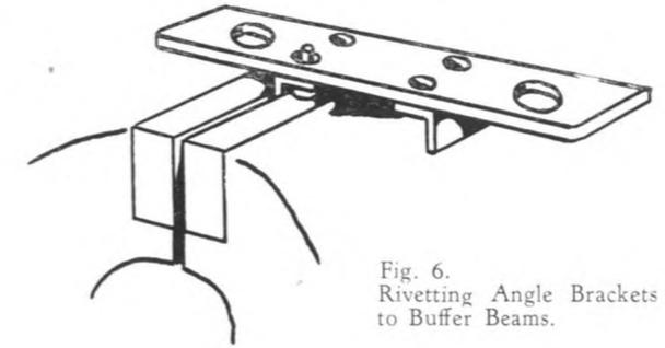
Fig. 6. Rivetting Angle Brackets to Buffer Beams.
