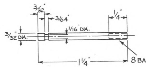
Fig. 71. The Valve Spindle.
