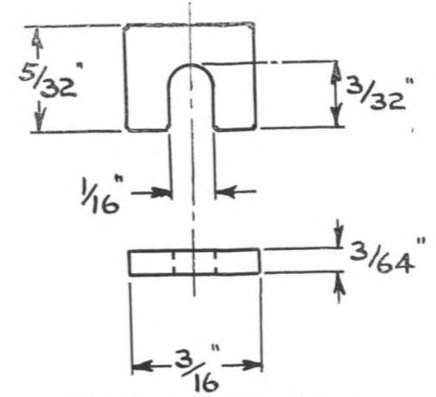
Fig. 72. The Valve Keeper.
