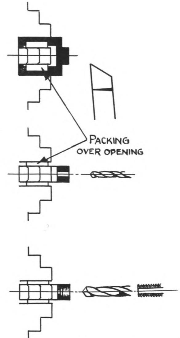
Fig. 68. Sequence of operations for machining end of steam-chest. (actual size.)
