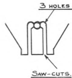
Fig. 4. Cutting Axlebox Slots.
