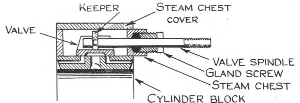
Fig. 73. Assembly of the Valve in the Steam-chest.
