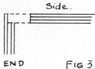
Planks are  $\frac{1}{10}$  in. wide on the main sides and the door planks are  $\frac{1}{12}$  in. wide. After the doors had been attached, the strapping was added as in Fig. 1.
