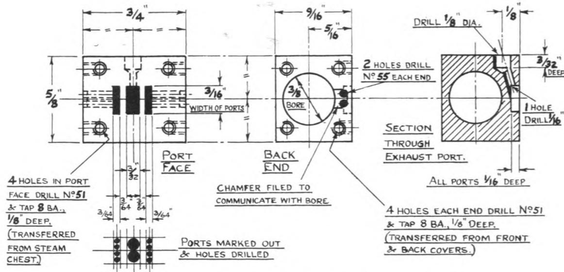
Fig. 50. The Cylinder Block.
