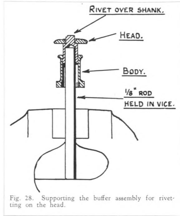
Fig. 28. Supporting the buffer assembly for riveting on the head.
