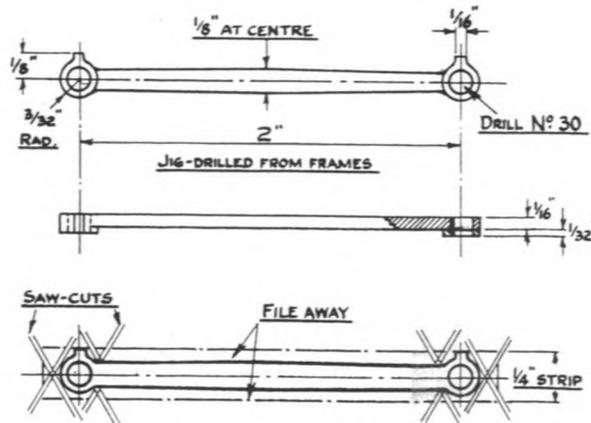
Fig. 47. Coupling rod, showing suggested method of cutting to shape. (Actual size 7 mm. scale.)
