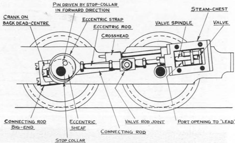
Fig. 87. The layout of the valve gear parts. (Actual size).
