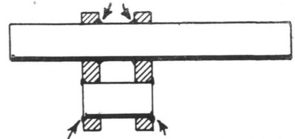
Fig. 38. Where to apply the silver solder.
