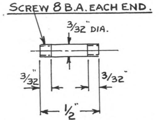
Fig. 80. The crosshead-pin. Material 3/32 in. silver-steel.
