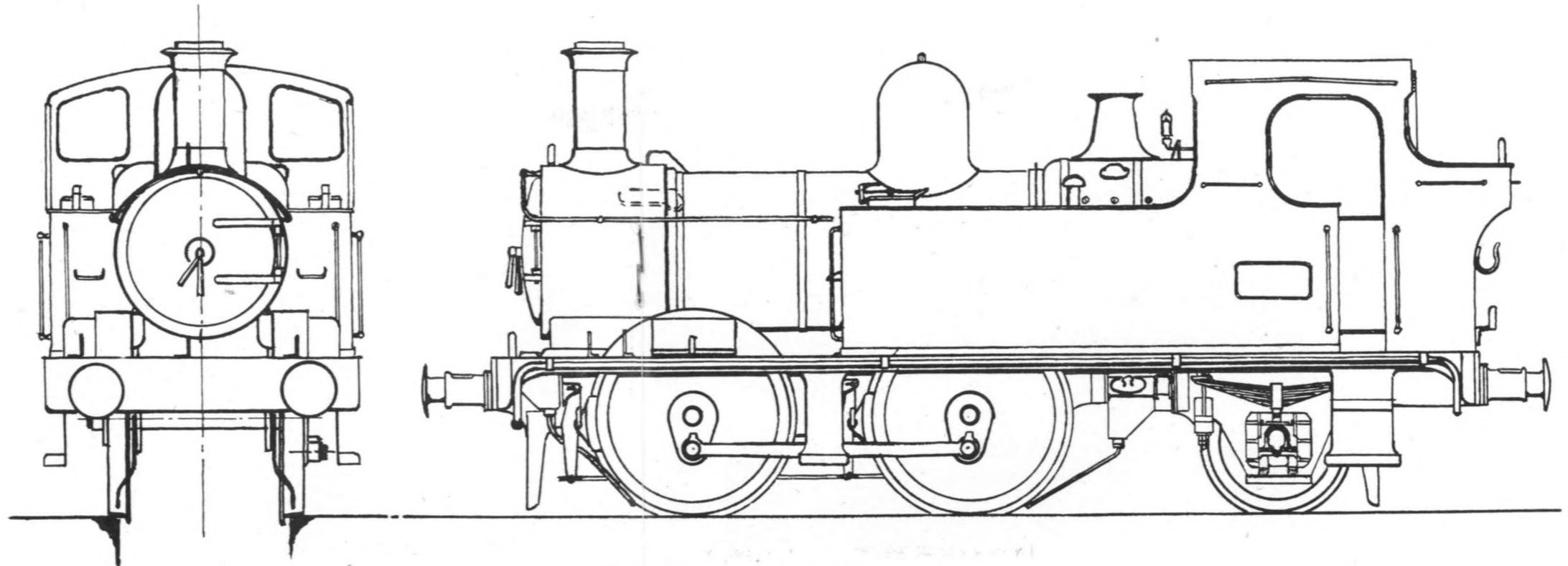
G.W.R. 0-4-2 TANK 1400 CLASS SIDE AND END ELEVATIONS.
