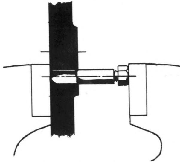
Fig. 34. Pressing crankpin into wheel.
