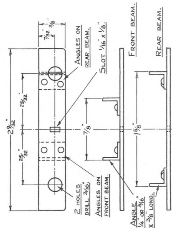
Fig. 5. Buffer Beams. Below: Photo—M. W. Earley.
