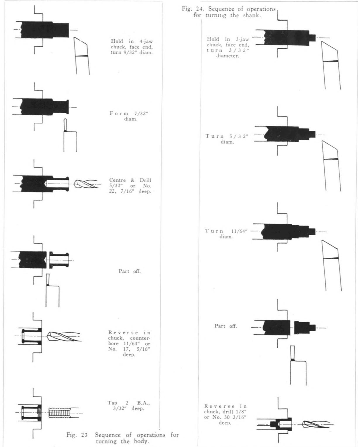
Fig. 23. Sequence of operations for turning the body.
