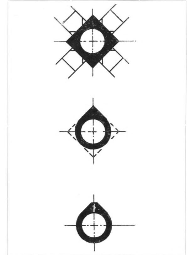
Fig. 41. Sequence of operations for making eccentric strap. Drawn full size. From top to bottom :
