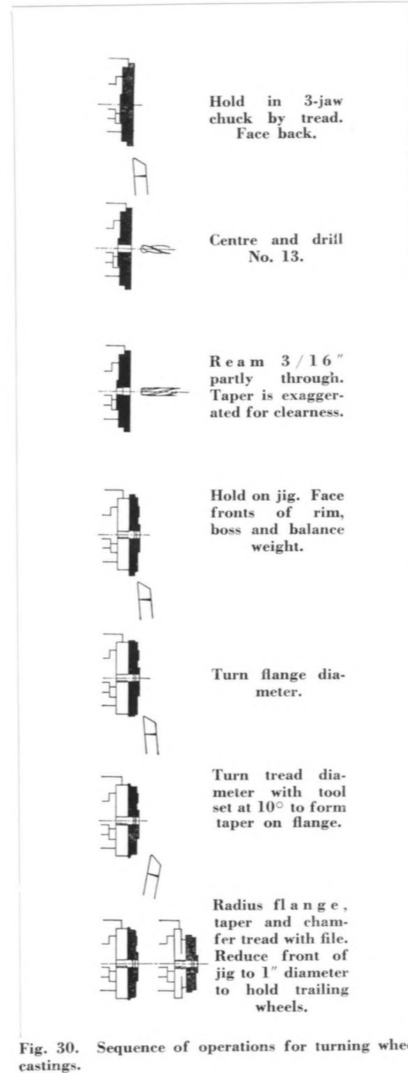
Fig. 30. Sequence of operations for turning wheel castings.
