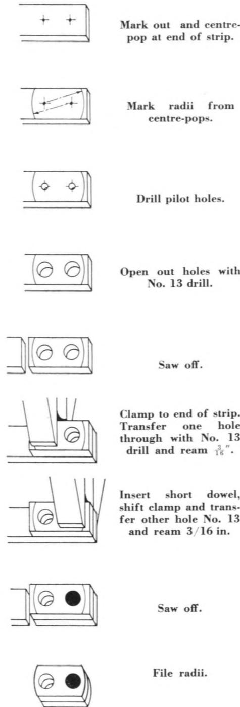
Fig. 36. Sequence of operations for making crank webs.
