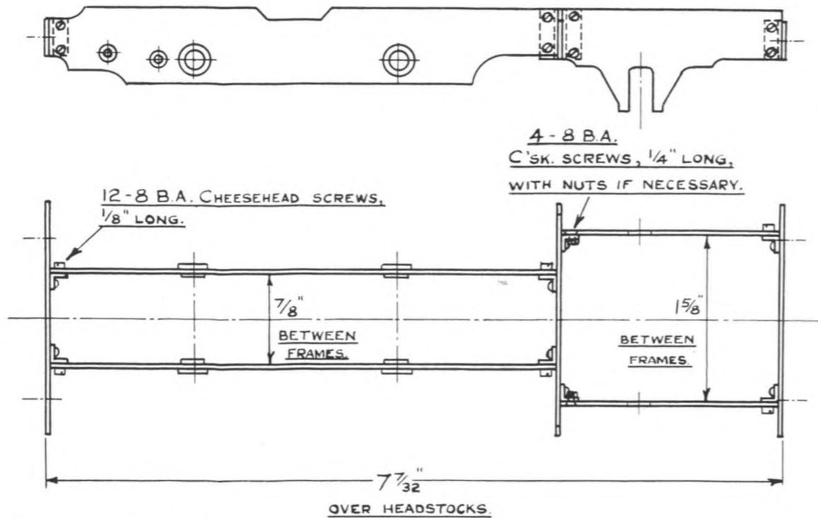
Fig. 11. The Frame assembly.
