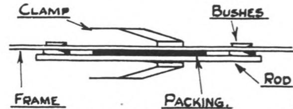
Fig. 45. Coupling-rod blank clamped to frame for spotting through.
