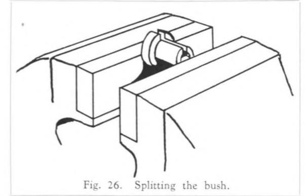
is, is put in and the whole lot tightened up together, the job should run as truly as if it were in a proper collet.
