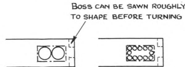
Fig. 67. Alternative methods of forming the opening in the steam-chest.
