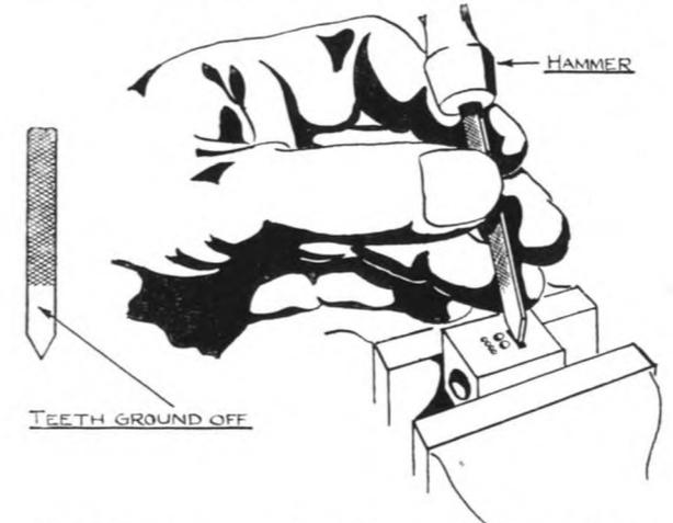
Fig. 52. A port-cutting chisel made from a broken piece of flat file and the chisel in use.
