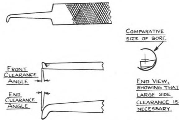
Fig. 51. A boring tool made from the tang of an old file.
