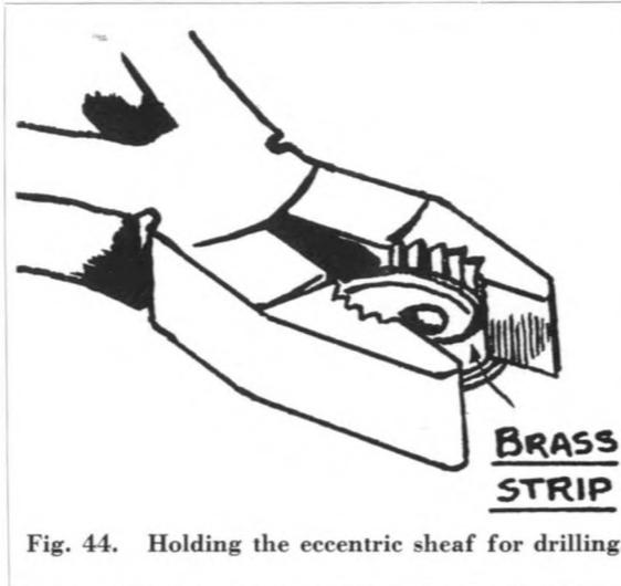
Fig. 44. Holding the eccentric sheaf for drilling.
